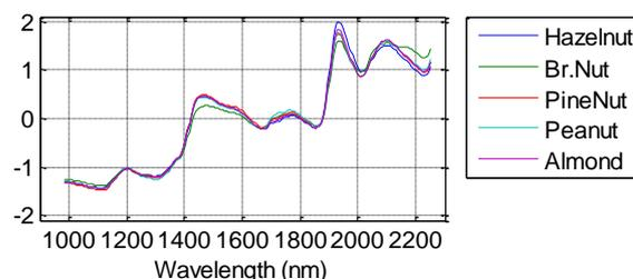
Fig. 3. Reference mean spectra of 5 nut contaminants. SNV pre-treated.
