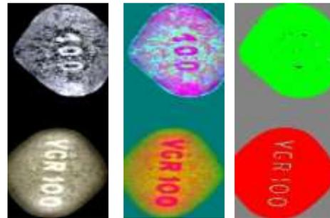
**Figure 1:** Images of the counterfeit (top) and genuine (bottom) Viagra® pills a) false RGB b) PCA c) classes
