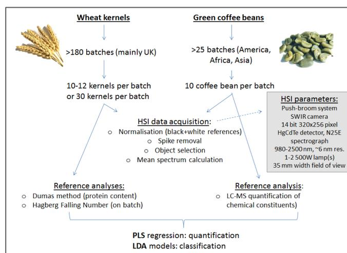
**Fig. 1.** Representation of the experimental plan for the present communication, regarding the application of HSI for the study of quality parameters in two commodities, *i.e.* wheat and coffee beans.
