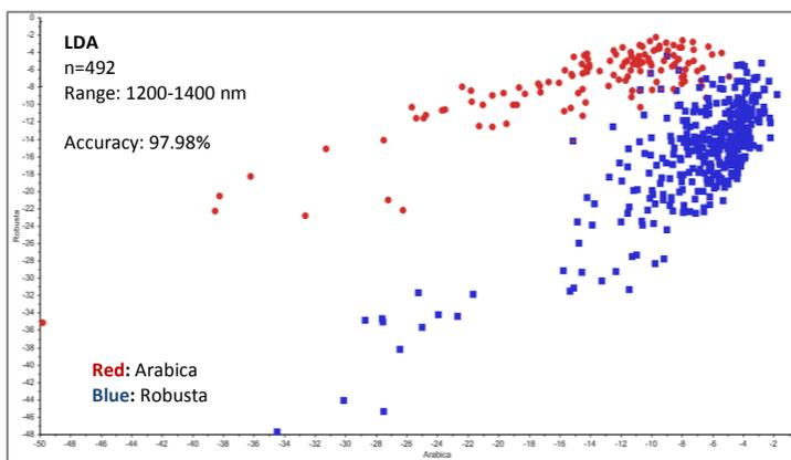
**Fig. 3.** Linear Discriminant Analysis (LDA) for green coffee beans Arabica/Robusta discrimination, based on HSI in the NIR region. Beans were scanned both on the ventral and dorsal side. Accuracy: 98.0%
