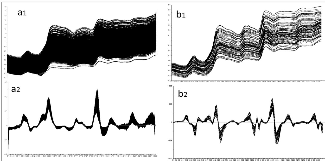
**Fig. 2.** Typical NIR absorbance spectra of: a<sub>1</sub>) intact wheat kernels, b<sub>1</sub>) green coffee beans; same spectra after first derivative calculation (a<sub>2</sub> and b<sub>2</sub>). Data were obtained at single kernel/bean level (mean spectra within the object).
