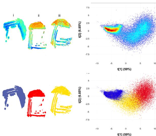
**Fig. 1** **a** PC1 score image of (i) *B. cereus*, (ii) *E. coli* and (iii) *S. enteritidis*; **b** score plot of PC1 vs. PC2 for the mosaic of *B. cereus*, *E. coli* and *S. enteritidis*; **c** score image showing bacteria coloured according to class membership, *i.e.* *B. cereus* (blue), *E. coli* (red) and *S. enteritidis* (yellow). **d** Projection of class membership onto score plot permitting easier visualisation of clusters.
