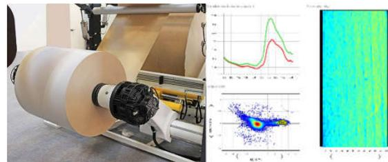
Fig. 1. Quantitative moisture profile mapping on paper rolls performed using RedEye HSI system in the 950 nm - 1700 nm spectral range.
