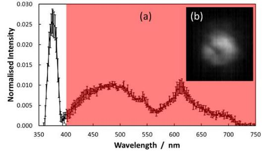
Fig. 5. (a) Average autofluorescence spectrum from small bowel tissue. The large peak is the 375 nm excitation light. (b) Fluorescence emission image using signal integrated from wavelengths greater than 400 nm.
