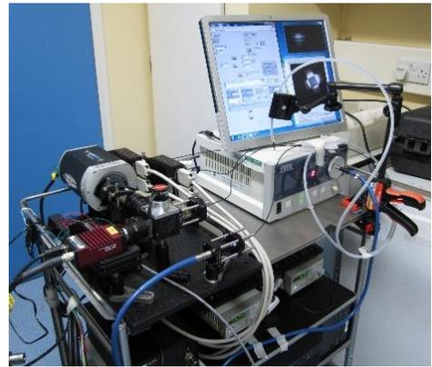
Fig. 1. Multimodal hyperspectral imaging endoscope.
