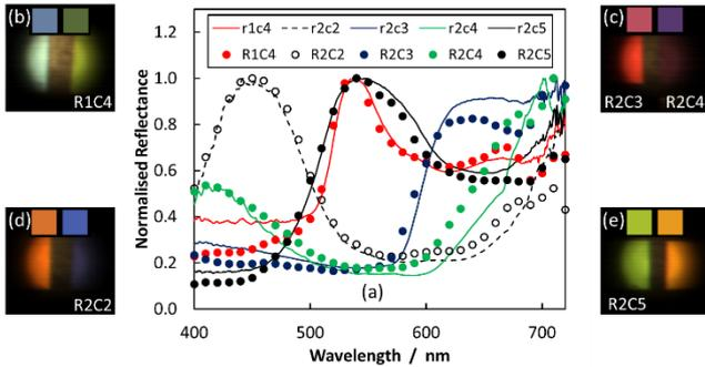
Fig. 2. Spectral validation. (a) Reflectance spectra of selected Macbeth panels measured using the HSI system (dots, 10 nm resolution) and stand-alone spectrometer (solid lines). (b-e) Corresponding reconstructed RGB images of panels alongside ground truth manufacturer images. *Modified from [7].*
